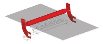
Martin<sup>®</sup> Pressure Roller Brackets provide firm support for the belt line over a secondary cleaner allowing effective cleaning. Available with new return rollers or use existing equipment. Mounts to conveyor stringer with three bolts or may be welded in place.
